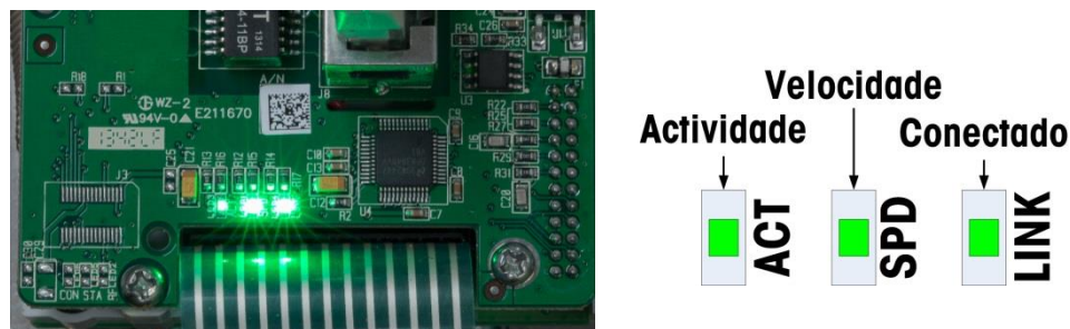
Figura 5-7: LEDs de Ethernet TCP/IP
