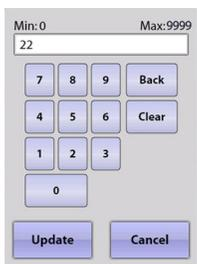
Touch the box next to “Mins” for a pop-up numeric keypad. Touch the **Clear** button on the keypad to delete the current value, and then use the numbers on the keypad to set the number of minutes of inactivity that must occur before Autoplay is activated. This delay time has a *minimum* setting of 15 minutes. After you have entered the time, touch **Update** on the keypad.
